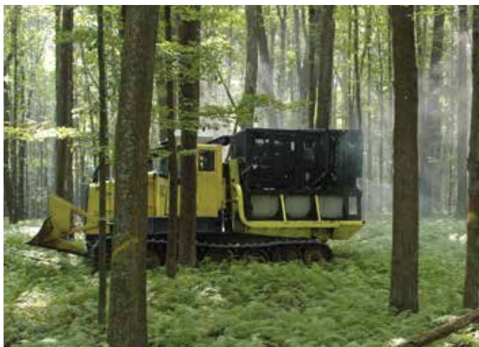
Tracked vehicle with an air-blast sprayer treating fern understory with an herbicide prior to harvest.
