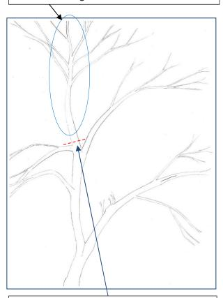
The final removal cut was made just above the union with a lateral branch.
